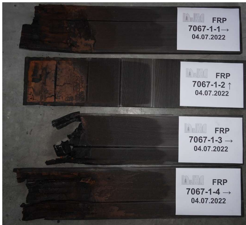
Fig.2. Test specimens after the test.
